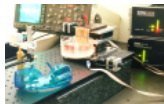
Figure 3: Measurement arrangement for transducer characterisation using a laser vibrometer and a positioning unit
